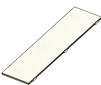
1X CEILING SUPPORT PANEL 780 SUPPORT CEILING
