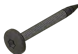
5 X F TRESPA SCREW T20 Ø4.8 L50 mm 637 048 050 T20 511
