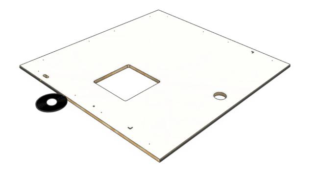
Cut & stick the provided adhesive strip of foam rubber on the edges of the ceiling panel. All the way around.
