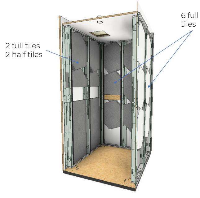
Fill the walls with the hexagon acoustic foam slabs. They need to be friction fitted at the top.
