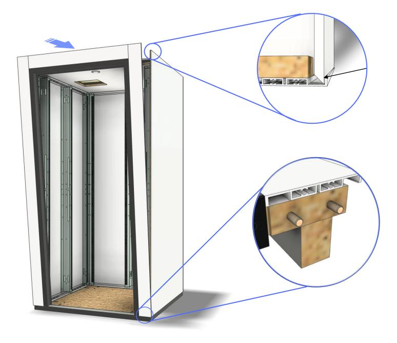
Mallet 4 wooden dowels in the bottom holes of the front frame.
