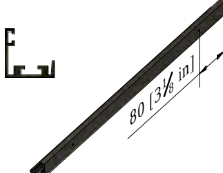
1X BOTTOM LEFT WINDOW BASE PROFILE. 570MM 731 HOR B 0570 L 501
